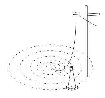
Positioning of the detector and its location relative to the voltage source can have a large effect on its sensitivity to electric fields.
