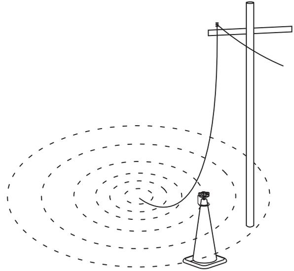
Positioning of the detector and its location relative to the voltage source can have a large effect on its sensitivity to electric fields.
