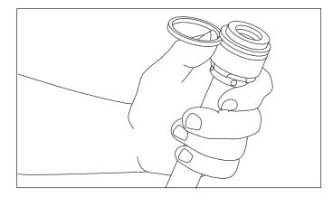
13. Bend the seal over as shown. This will help hold the seal in the groove when installing.
