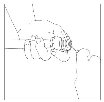
18. The piston seal will be stretched out of shape when installed in the groove. Place the piston with the seal installed on a clean, flat surface and roll it back and forth to reshape the seal.
