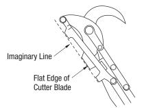
When closed, the blade should cover 5 mm (3/16") on the face of the cutter hook.
