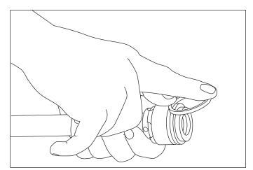
14. Remove the seal from the groove.
