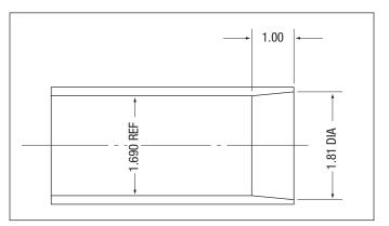
20. Lubricate the tapered fixture end with oil or grease.
