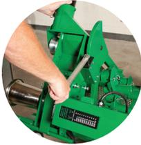
**1** Lift the boom to desired angle using crank
