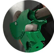
**3** Position the nose just over conduit and lower adapter into conduit by cranking the boom lower
