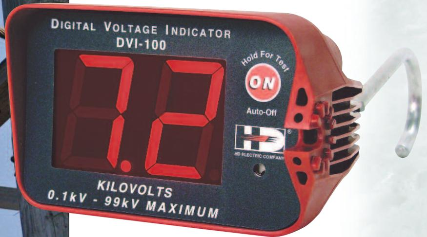
The DVI-100 is designed to be used on distribution systems in both overhead and underground applications and on transmission systems up to 161kV. The DVI-100 indicates voltage from 0.1kV – 99kV and is auto-ranging. Voltage is displayed on a large 2.25" LED display with a 2-digit readout. In addition, an audible alarm alerts the user to the presence of voltage above 100VAC. The DVI is auto shut-off and will turn off after 3-4 minutes of inactivity.
