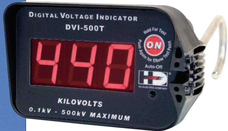
The DVI-500 is designed to be used on both transmission and distribution systems in overhead and underground applications. The DVI-500 indicates voltage from 0.1kV – 500kV and is auto-ranging with no range selector switch or settings required. Voltage is displayed on a large 1.45" LED display with a 3-digit readout. In addition, an audible alarm alerts the user to the presence of voltage above 100VAC. The DVI is auto shut-off and will turn off after 4 minutes of inactivity.
