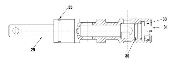
Figure 4 Spool shown in Closed-Center Position
