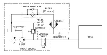
Figure 2 Hydraulic Schematic
