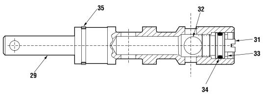
Figure 8 Spool shown in Open-Center Position
