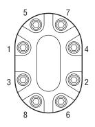
Figure 3 Torque Sequence
