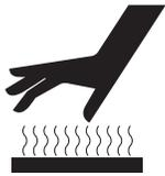
Tool and accessory may be hot during and after operation. Allow to cool before handling, or handle with heat-resistant gloves.
