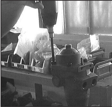
8. Loosen the four screws on the accumulator.
