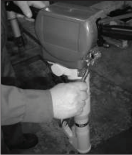
1. Loosen the screws to remove the top cover.
