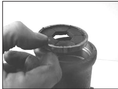
5. Remove the chisel bellows.
