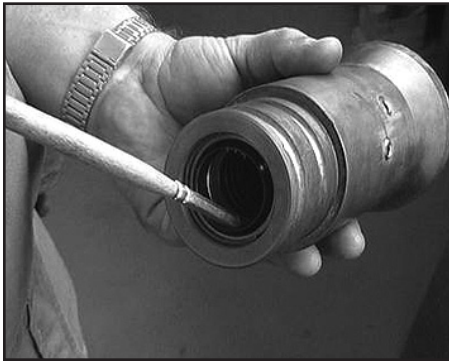
1. Oil the seals in the cylinder.
