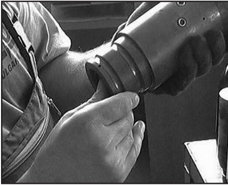
9. Check the movement of the striking piston.
