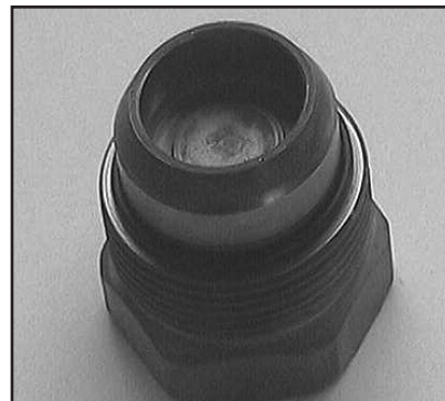
5. Grease and mount the O-ring on the T guide socket.
