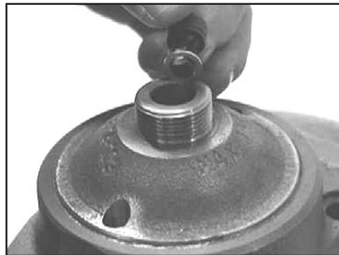
7. Mount the charging screw and seal ring.
