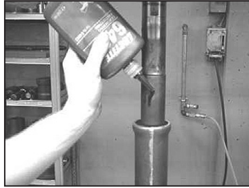
4. Apply Loctite 648 to the bushing.
