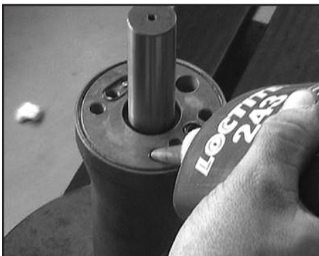
4. Apply Loctite 243 (245) to the cylinder thread.
