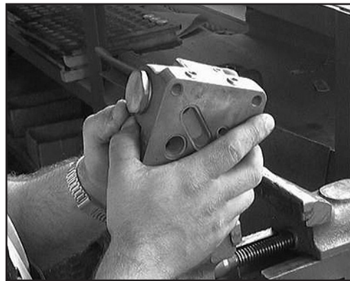
13. Check the movement of the spool by shaking it from side to side.
