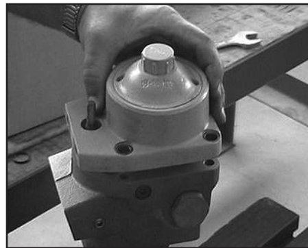
15. Mount the accumulator.
