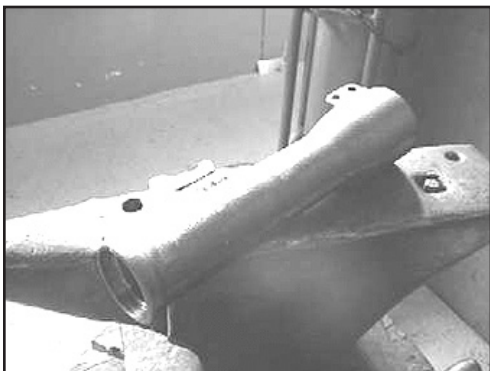
4. Place the nose part on an anvil.
