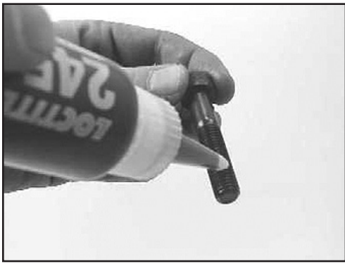
18. Apply Loctite 245 to the screws.
