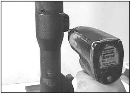
2. Loosen the nose part with a drill or torque wrench.
