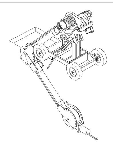
Pulling Horizontally in Manhole Using Two Booms, Nose Unit, Elbow Unit and Slip-in Coupler
