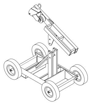
2. Set puller on boom mount frame so that the puller mounting feet sit inside the frame opening, between the two side rails. Slide the puller up against the stop and chain it down securely.
