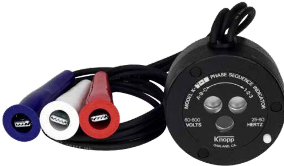
The K-7-1 Phase Sequence Indicator indicates the order of succession in time of the different voltage peaks of a multi-phase supply. The K-7-1 is used to make three-phase circuit installations or alterations as well as replacement installations of motors and generators. It can be used for making continuity tests of circuits of poly-phase systems. It is also valuable in making connections of power-factor meters, voltampere meters, watt and watthour meters and relays.
