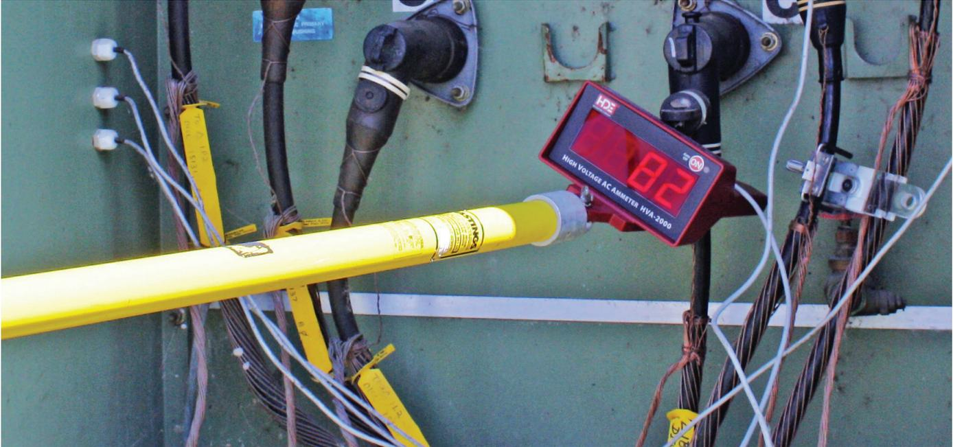
Primary voltage cables are generally shielded and the Ammeter cannot measure current on a shielded cable except in areas where the shield has been removed.
