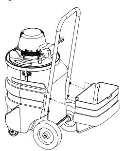
3. Attach the storage box lid to the handle by using two shoulder screws (47) and two nuts (48).
