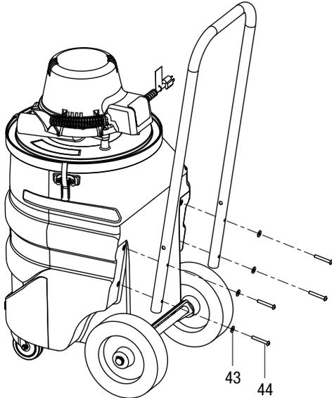
2. Attach the storage box to the tank by positioning the box over the screws and washers from the handle and sliding the box down firmly until it locks into place. If preferred, tighten the screws to squeeze the storage box. Be careful **NOT** to overtighten.
