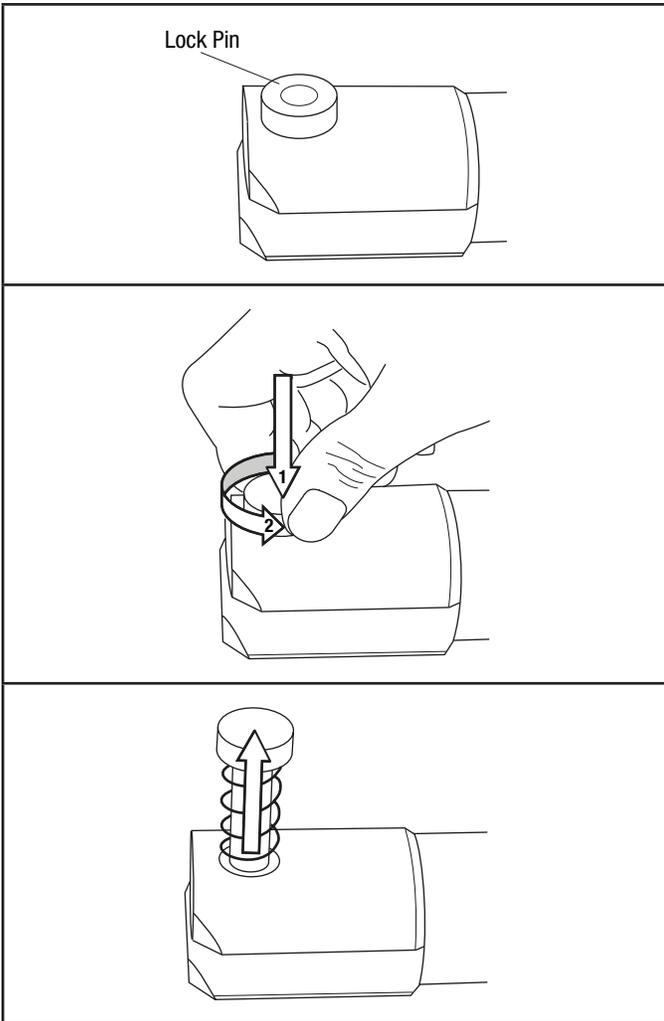
4. Install the jaw into the pressing tool and align mounting hole in jaw with lock pin. Depress the lock pin to secure the jaw (see views below).
