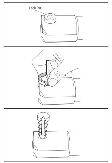
4. Install the jaw into the pressing tool and align mounting hole in jaw with lock pin. Depress the lock pin to secure the jaw (see views below).
