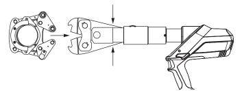
12. Disengage the release pin on the pressing chain and remove the pressing chain from the pressed fitting.
