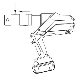
Note: Rollers must be in the forward position to allow the sleeve to be moved to the corrrect position.
