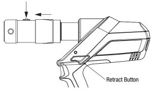
4. Depress retract button to retract rollers to the back position or complete a trigger cycle to achieve same result.
