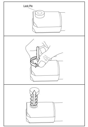
6. Install the adapter jaw into the pressing tool and align mounting hole in jaw with pin. Depress the pin to secure the adapter jaw (see views below).
