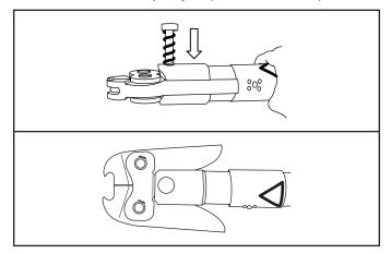
7. Compress the ends of the adapter jaw together to open the jaws and install the adapter jaw into the pressing chain (see view below).
