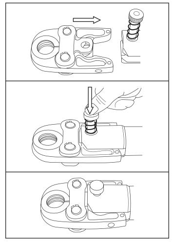
5. Compress the ends of the jaw together to open the jaws and locate the jaws around the fitting to be pressed (see view below).
