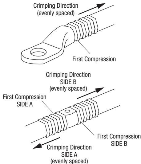
7. Using the sequence illustrated here, press the trigger to advance the dies. Continue to crimp until the pressure relief valve activates.
