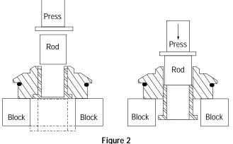
Figure 2 Bearing Removal
