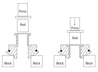
Figure 3 Bearing Installation
