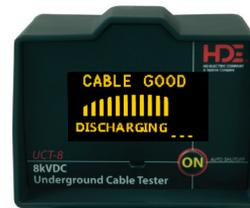
Good cable test results - cable discharging
