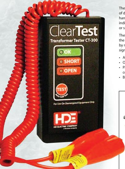
The ClearTest Transformer Tester provides quick and easy tests of de-energized power distribution system transformers. It is a handheld device with a single pushbutton that provides a clear indication of open circuits, short circuits, including shorted turns or shorted windings and confirmation that the test results are OK.
