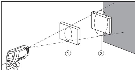
Object 1 is the correct distance from the unit. Note the target is slightly larger than the spot size being measured.
