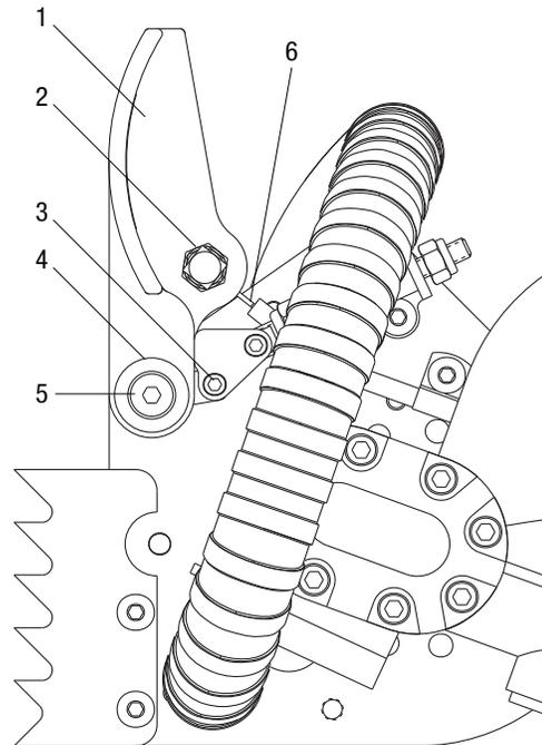
1. Loosen bowden pin (2) to release cable (6).
