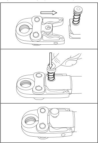
4. Compress the ends of the jaw together to open the jaws and locate the jaws around the fitting to be pressed (see view below).
