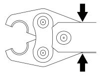
Reinstall the battery and depress the tool trigger to press the fitting. Continue to depress the trigger until the relief valve actuates and the drive rollers automatically retract.
