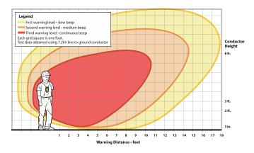
Conductors of different phases in close proximity will also reduce warning distances due to field cancellation effects.
