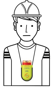
When the V-Watch Personal Voltage Detector is in use with a good working battery, it is always on, always ready to warn of potentially hazardous high voltage. The battery life is approximately six months of continuous use or two years in storage. When the job requiring the protection of the detector for the user is completed, the detector should be closed by pushing down on the top.
