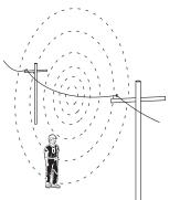
a high voltage field surrounding the conductor that the detector will sense and warn the user.
