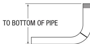
Measure and mark the length of the stub. Subtract the radius of the bend and 1/2 of the O.D of the pipe. Add 1/2 of the developed length.
