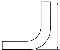
16. **rise** — the distance from the end of a vertical section of conduit or pipe to the bend; measured to the outside edge of the conduit or pipe
