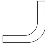
11. **90° bend** — any bend that changes the direction of the conduit or pipe by 90° degrees
