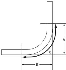
7. **gain** — because conduit and pipe are bent with a radius and not at right angles, the length of conduit or pipe needed for a bend is less than the straight-line measured length; gain is the difference between the right angle distance (A + B) and the shorter curved distance (C)
