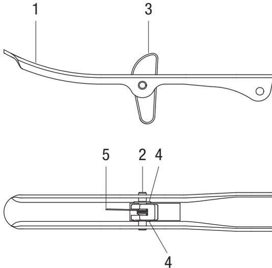
1. Position the trigger (1) and safety latch (3) as shown.
