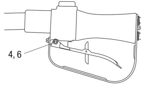
5. Remove the retaining ring (4) and trigger pivot pin (6), which secures the trigger interlock assembly. Remove and discard the trigger assembly, trigger pivot pin, and retaining rings.
