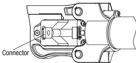
3. If open, close the crimping head. Make sure the head and latch are fully engaged.
