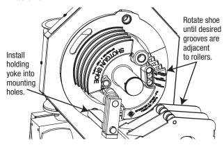
Load the conduit so that the bending mark is aligned with the front edge of the holding yoke, as shown.
