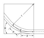
**developed length** — the actual length of pipe that will be bent; refer to distance "d" in the illustration at left.
