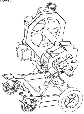
2. Slide the shotgun bending shoe onto the shaft of the main sprocket, as shown. Align the four drive studs on the back of the shoe with the four holes in the main sprocket. Make sure to align the drive stud with the cap with the bigger hole on the bender.
