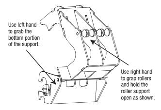
2. Align the right plate of the support with the bender roller plate as shown in the steps below.
