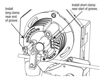
4. Slide a piece of scrap conduit, square tube, or bar through the two clamps and tighten the clamp screws. Make sure the back of the conduit is shorter than the shoe radius. 5. Slide the stopper assembly onto the tube or bar until the stopper contacts the conduit and tighten the clamp screw, as shown.
