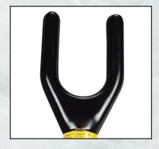
The fork style sensing head has been designed to help facilitate taking measurements in underground (U/G) applications. It can be used in other applications including overhead (O/H). Outside head dimensions are 5.5"W x 8.5"L x 1.1875" Thick (14 cm x 22 cm x 3 cm). Inside head dimensions are 2.75"W x 5.5" Deep (7 cm x 14 cm). For ordering, please refer to model numbers 8281 and 9391 in the Ordering Information box.
