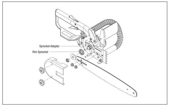
Figure 16 Rim Sprocket and Sprocket Adapter
