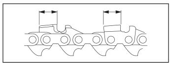
5. File enough to remove any damage to the cutting edges (side plate and top plate) of the cutter.
