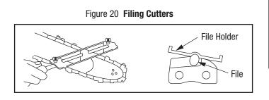
2. File the cutters on one side of the saw chain from the inside out. File on the forward stroke only.
