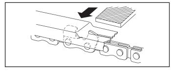
4. See Figure 19. Round off the front corner to maintain the original shape of the depth gauge after using the depth gauge tool. Always follow the recommended depth gauge setting of the chain manufacturer. This is important for maximum performance throughout the saw chain's life as well as for protection against kickback.
