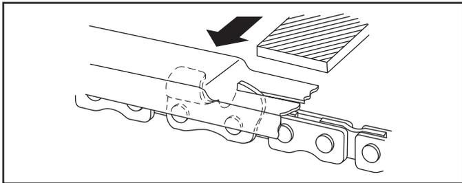
4. See Figure 19. Round off the front corner to maintain the original shape of the depth gauge after using the depth gauge tool. Always follow the recommended depth gauge setting of the chain manufacturer. This is important for maximum performance throughout the saw chain's life as well as for protection against kickback.
