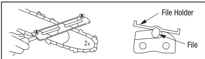
2. File the cutters on one side of the saw chain from the inside out. File on the forward stroke only.
