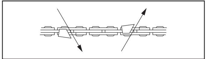
3. Keep the line on the file holder parallel to the center of the saw chain. Reverse the procedure for the other side.
