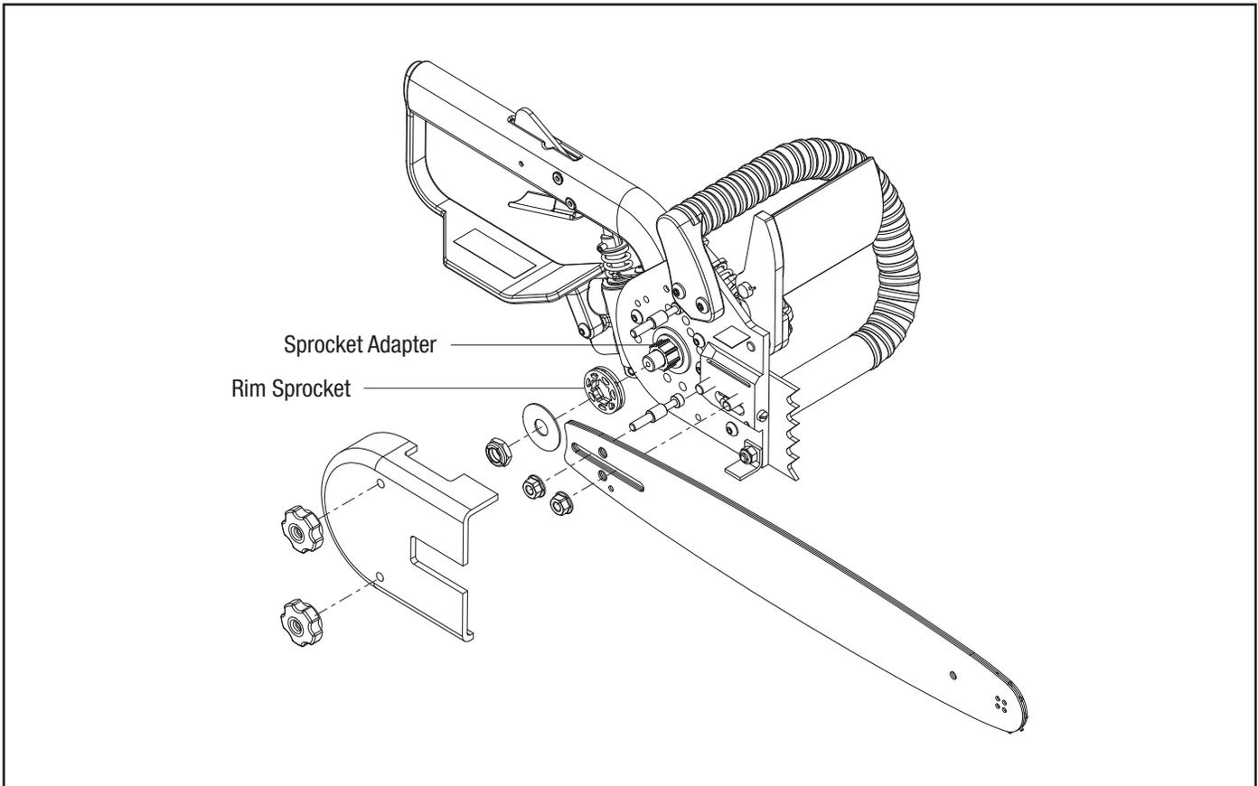
6. Use the mark made in Step 1 to install the bar upside down, so that the bar will wear evenly.
