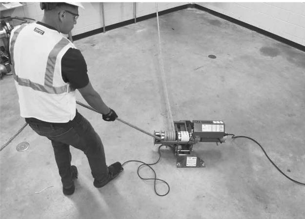
**Figure 31: Proper Operating Position Floor Mount**
