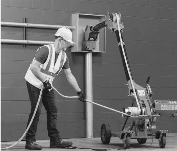
**Figure 30: Proper Operating Position MVB**
