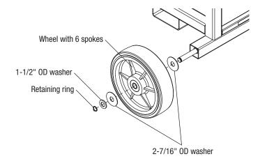
Wheel assembly is correct. No rework is required.
