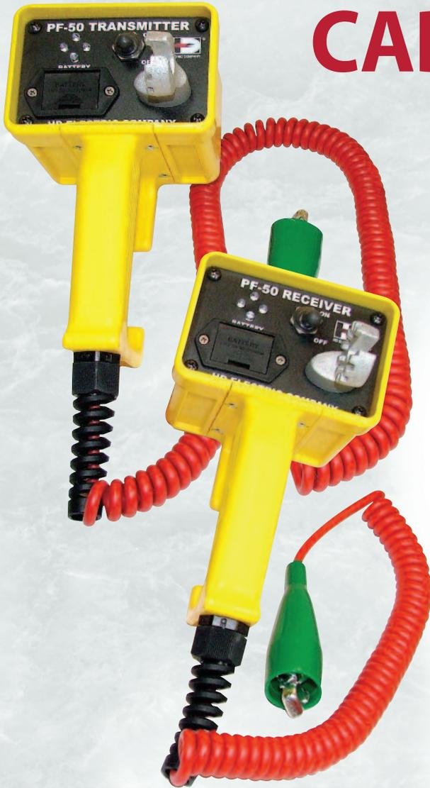
The PF-50 Cable Identifier identifies the correct phases of de-energized and discharged overhead and underground cables. It consists of a transmitter and receiver that are designed to be hand held with or without gloves or with optional accessory hotsticks. Red LED's on both units indicate that the PF-50 units are connected to the same cable. Maximum cable length is 5,000 feet. Because of its higher test voltage, the PF-50 can test a mile of cable.
