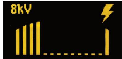
If the cable leakage current drops to near zero, the CABLE GOOD message will be displayed and the cable discharging current is now shown in the bar graph.
