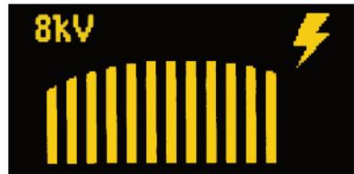
The presence of high voltage DC from the UCT-8 is indicated by the lightning bolt symbol at top right of the display.
