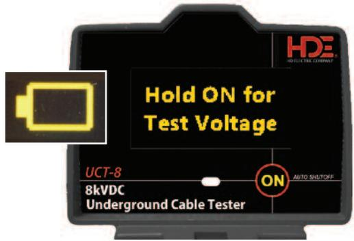
In the event the UCT-8 is connected to a live cable energized with 50/60Hz AC voltage, that voltage will be displayed on the front panel and testing cannot proceed until the cable is verified deenergized. This cable should also be grounded to completely discharge it before beginning the test.
