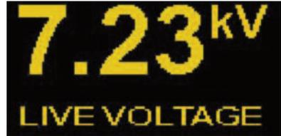
If no AC voltage above 100V is detected, the UCT-8 is ready to test the underground cable.
