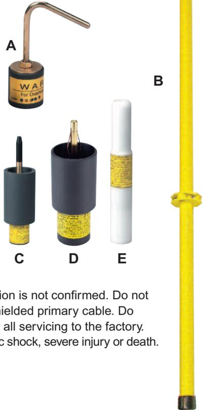
**WARNING:** Do not use the UCT-8 if proper operation is not confirmed. Do not use it to test equipment other than underground shielded primary cable. Do not apply to energized circuits or equipment. Refer all servicing to the factory. Failure to follow these instructions may lead to electric shock, severe injury or death.
