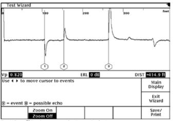
TestWizard<sup>™</sup> Testing automatically marks faults.
