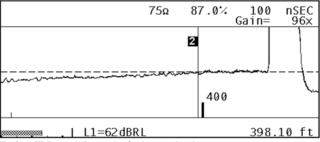
Typical TDR test misses the fault completely.
