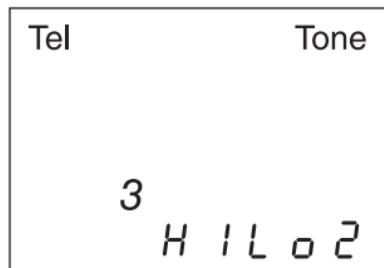
In this screen only wire "3" of the telephone cable is carrying the "HiLo2" tone.
