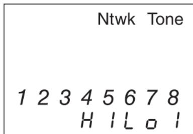
This screen shows, for example, that all wires of a network cable are carrying the "HiLo1" tone.
