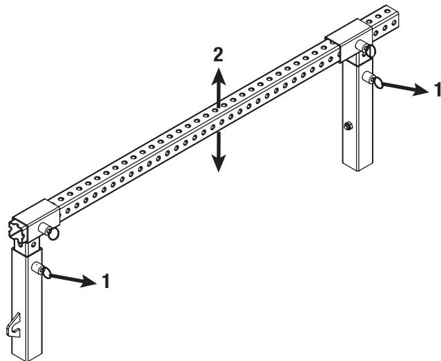
6. Mount the feeder according to which direction the cable is to be fed by disengaging the pull pin and setting the feeder on the cross bar. Slide the feeder along the cross bar to the desired position to feed cable. Be sure that the pull pin properly engages into a hole on the cross bar.
