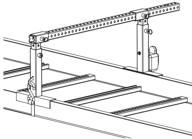
5. **CTF-200EXT only:** Adjust the height of the cross bar (2) using the pull pins (1) from the lower mounting legs.
