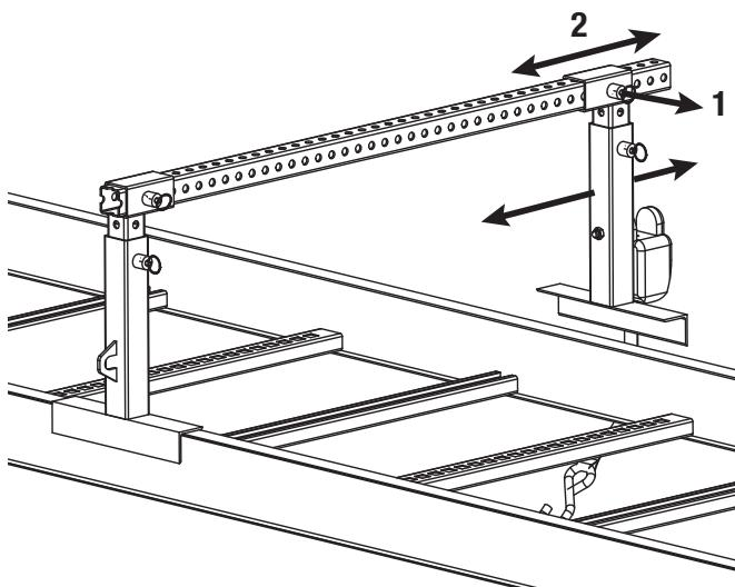
3. Draw out the strap from the ratcheting mechanism and hook to the opposing leg hook.
