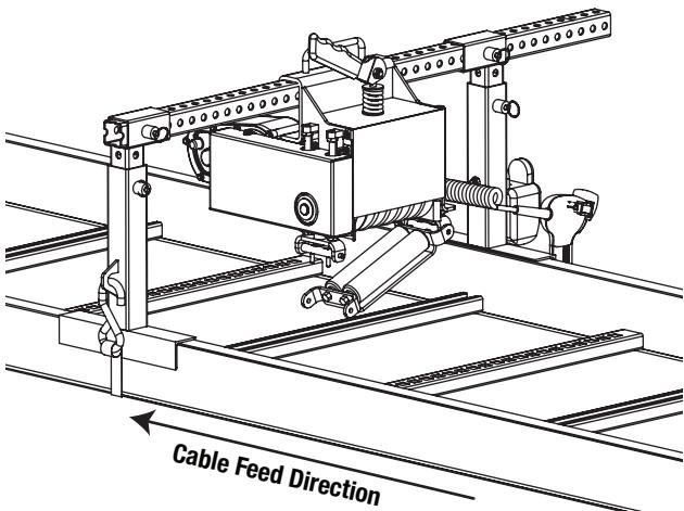
2. Plug in the device to any standard 115 VAC circuit (refer to "Grounding Instructions"), and plug in the pendant to the jack labeled pendant. Switch main power to ON.
