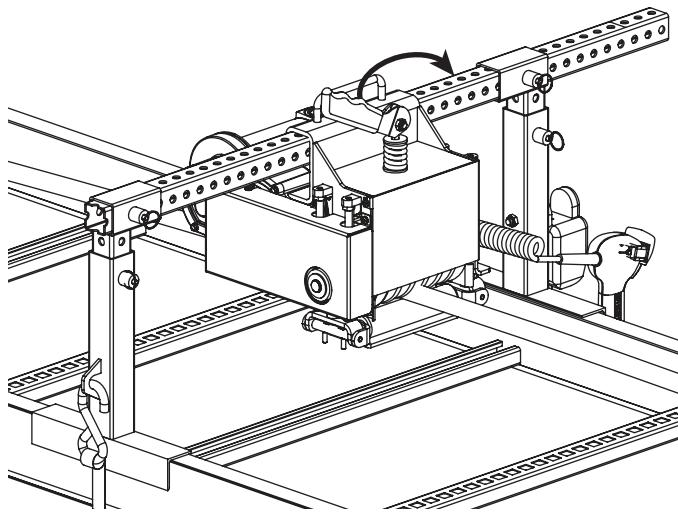
4. Activate the feeder by continuously pressing the pendant rocker switch. Starting with the speed at the lowest point, bring the speed up to match the speed of the puller.
