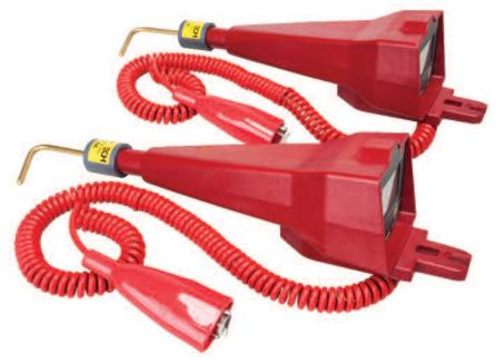
The high voltage resistors limit the current through the ground cord to a maximum of less than one milliamp. Although the ground cords are insulated for voltage up to 20kV, they should always be kept free and clear from you and any other conductors.
